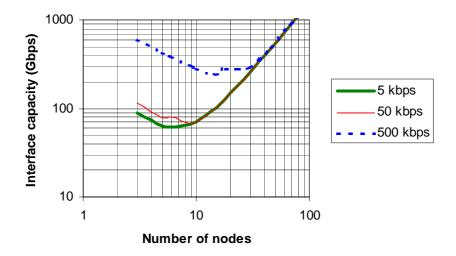
Fig 4. Total interface capacity of one router as a function of the number of core nodes. 5, 50 and 500 kbps = average traffic generated by one user, 1 000 000 users.
