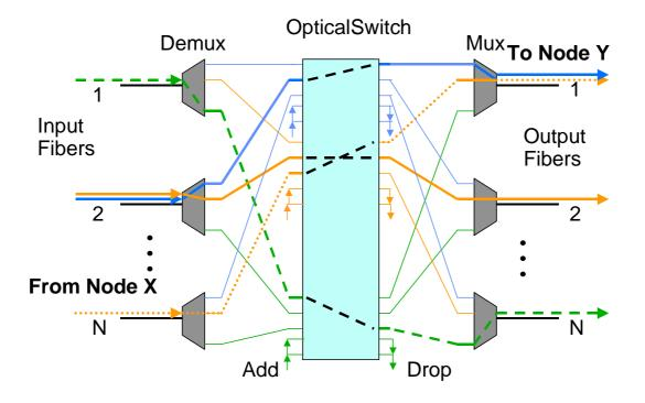
Fig. 2. Optical Wavelength Router node description. E.g. The dashed wavelength from input fiber 1 is routed to the output fiber N. Typical number of fibers ('links'') could be 4..16 including the local add/drop ports. Additional to the figure Interface boards with transmitter/receiver, optical amplifiers and a control system need to be installed.
