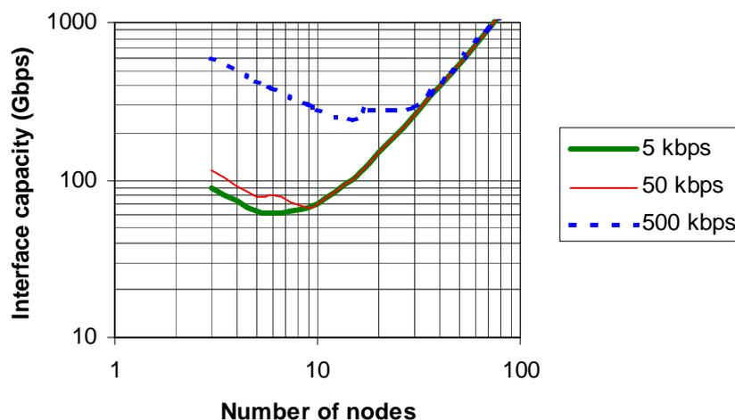
Fig 4. Total interface capacity of one router as a function of the number of core nodes. 5, 50 and 500 kbps = average traffic generated by one user, 1 000 000 users.
