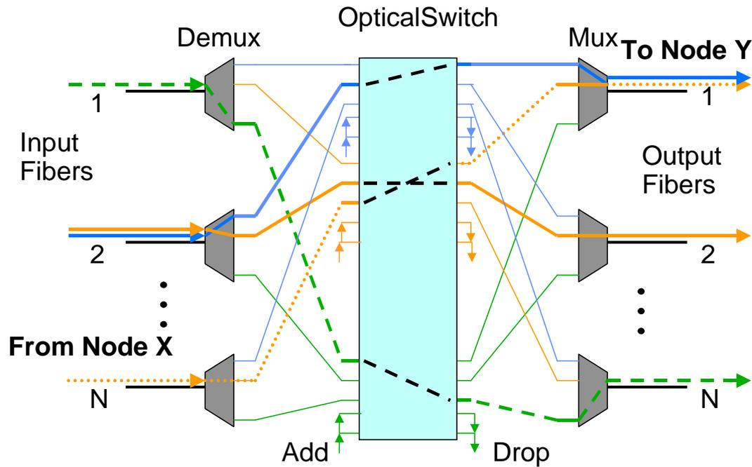
Fig. 2. Optical Wavelength Router node description. E.g. The dashed wavelength from input fiber 1 is routed to the output fiber N. Typical number of fibers ('links') could be 4..16 including the local add/drop ports. Additional to the figure Interface boards with transmitter/receiver, optical amplifiers and a control system need to be installed.
