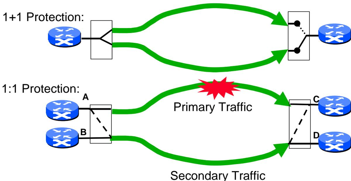
Fig. 3. Protection principles in the optical layer. In a wavelength router, the protection is put between two end nodes of the light-path. Thus, both the primary and protection signal can traverse several Wavelength router nodes.
